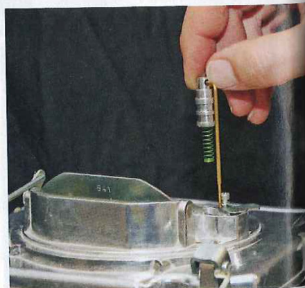
◆ Metering rods are easily accessed, the same way they are on an AFB-style carburetor. Metering rods are two-step design.
