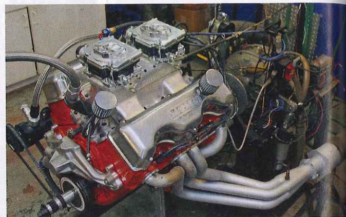
◆ On the dyno, the Street Demons made more power than modern AFB-style carbs on a hot street 409 engine. Showing these carbs are excellent for all-out performance applications, Walden got the first two 750-cfm carbs for a 509-inch 409 race engine with original high-port Z-11 heads. Walden built the engine with an original Z-11 intake and modern AFBs, and ran out of carb. After adding a pair of 625-cfm Street Demons, they ran out of intake, so they bolted on one of their own intakes, ran out of carb again, and added the 750-cfm Demons—when it was done, they'd picked up more than 100 hp over the high-zoot factory mini-tunnel ram and modern AFBs—which was previously one of the best combos available for a 409.
