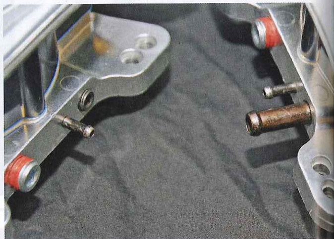
◆ When running them as a dual-carb setup, Walden found the vacuum port needed to be removed and the hole plugged.
