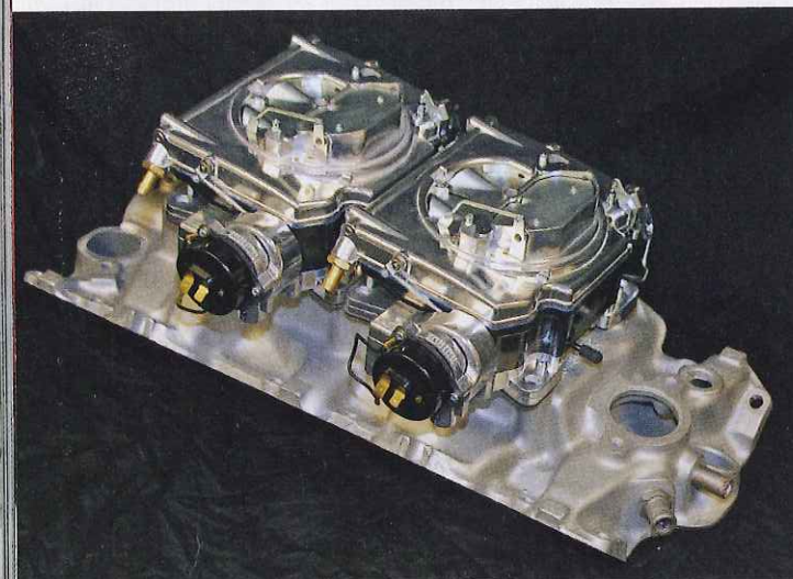
◆ This is one of the great aspects of the Street Demon carbs—unlike regular Holley carbs, these will bolt to factory GM 2x4 intake manifolds. Previously, only modern AFBs and original carbs could be used due to spacing.
