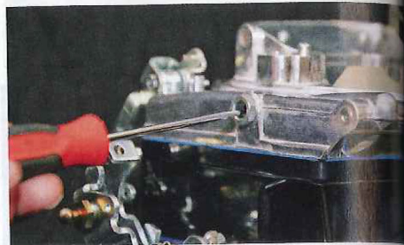
◆ The secondary air valve control is spring loaded, and fully adjustable—a screw and locking nut allow you to tune the tension on the torsion spring for primary-to-secondary throttle “tip-in”, independent of the throttle-opening rate.
