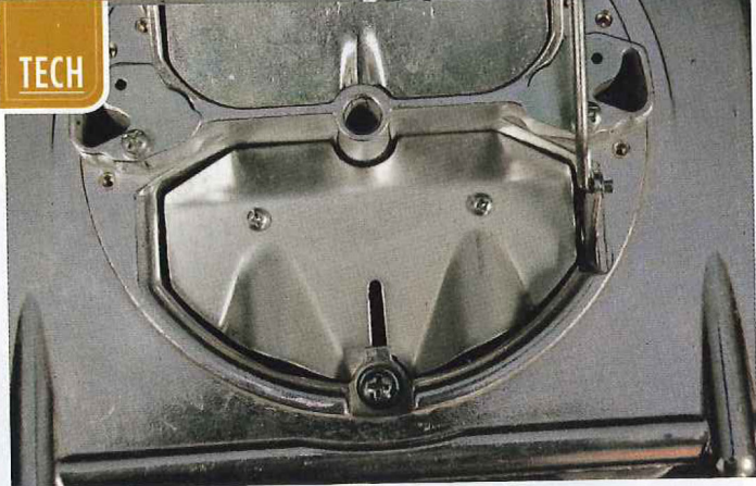
◆ The secondary air valve control is spring loaded and vacuum operated.
